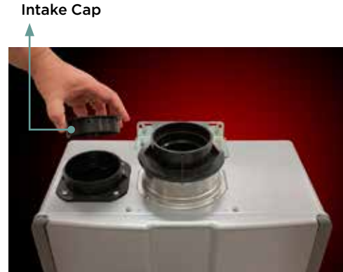
For PVC/CPVC configurations, the intake cap is removed and discarded. With this option, installers can use three- or four-inch PVC/CPVC pipe for the intake and exhaust.
